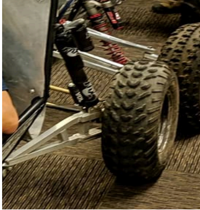
Figure 3 - Car 44's rear suspension design. [2]
