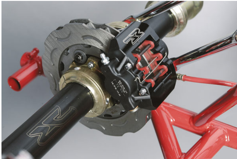
Figure 34 - Slotted and Ventilated Rotor with Fixed Caliper
